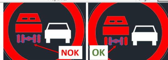
IMPORTANT: All the areas of the sign must be covered by hatches. Do not leave any space without hatch.
